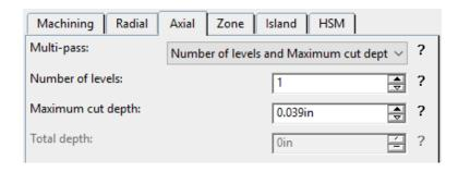
Multi-pass Defines how the multiple axial steps are calculated
