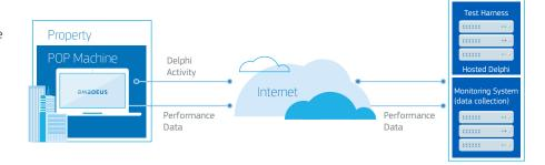
(POP machine) that communicates to the hosted environment (test harness) over the Internet and executes predefined application actions. Data is continuously collected on the performance of these actions. At the conclusion of the five-day monitoring period, Amadeus will present a data analysis report.
