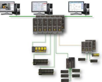
The VE6042 or VE6043 can also be used as a central switch if a more modular switch solution is required or to meet extended environment specifications due to the location of the central switch.
