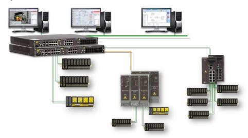
Typical network implementation would use the VE6048 as a central switch located in a rack room where AC power is available with the VE6041 (or VE6042 or VE6043) as a field-mounted switch for controllers in field-mounted locations. If required as part of the network architecture, multiple VE6048 switches can be interconnected using the gigabit ports to provide a network backbone to connect devices or other DeltaV switches.
