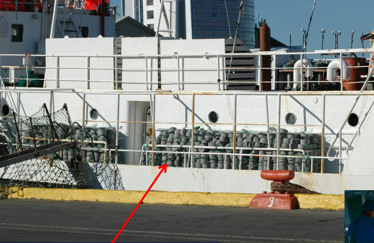
Concrete cylinders, Chilean longliner, K. Dietrich 2010
