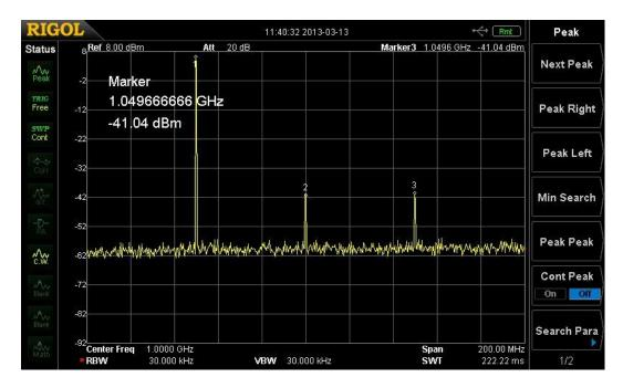
So again a Band pass filter is attached to the PA but now on the output side. Reason is of course that if you transmit these frequencies thru the antenna you will generate disturbing signals to all other RF
