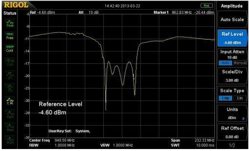
Add. Info: Why does the band pass filter looks as it look? In the pass frequency range of the filter should be maximum matching to 50 Ohms, so that all frequencies which are in this region can pass the filter without too much loss. Outside there is maximum "unmatch" so that the frequencies will be reflected. What we see on the screen is that in the pass region less signals are reflected and being measured by the DSA.
