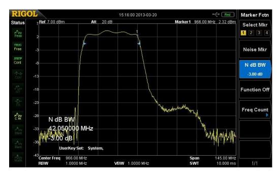
The 3dB Bandwidth of the filter is around 42MHz. If you would like to measure the input attenuation of your filter you have to perform Normalization before starting the measurement. The Normalization can be done under TG menu structure.
