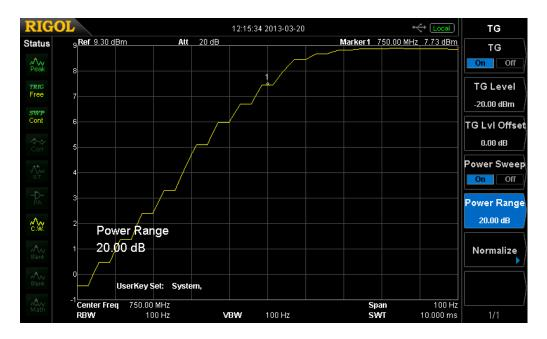
We now see on the screen the change over from the linear behavior (to marker) to the non-linear range of the PA. The point when the measured power differs 1 dB from the theoretical linear extension is called the 1dB-compression point and this is a very important parameter in PA specs.
