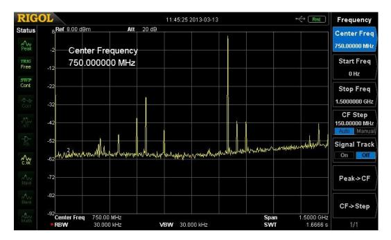
You can see that there again occur a lot of unwanted frequencies. They are generated from the unlinearities of the PA and also the still existing low power peaks from the mixing stage are amplified with 20dB and arise again.
