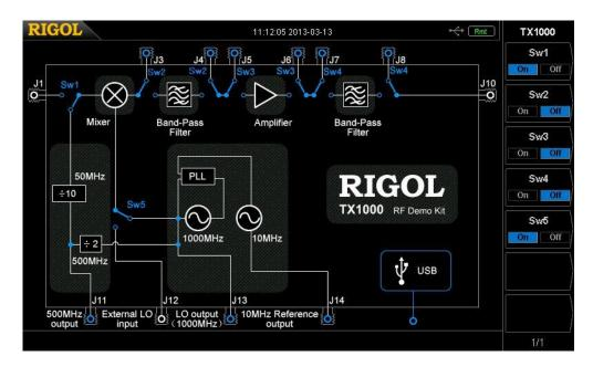
Above you see the screen shot of the TX1000 control which is built in the DSA815. To get the same picture first connect your TX1000 thru USB to your DSA815(-TG). Press System -> go to page2 -> TX1000 and you should see the control user interface. For the first measurements please set it as seen above and connect your DSA Input to J3 connector of your TX1000.
