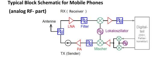
The schematic above shows a typical front end of a mobile phone. Our TX1000 RF Demo Kit shows has the same setup as the TX path of the Mobile Frontend. Mixer (Mischer) -> Band pass filter -> Power Amplifier (PA) and again a Band pass filter on the output to the antenna. Only difference is, that at the filter at the antenna of the Mobile Phone is a Diplexer which also split RX and TX frequency bands.
