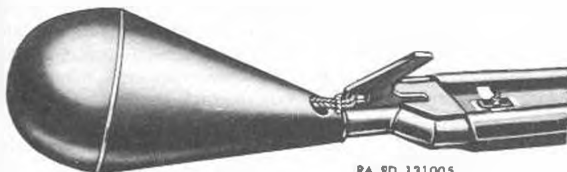
Figure 87. Nose assembly, demolition snake M3.
