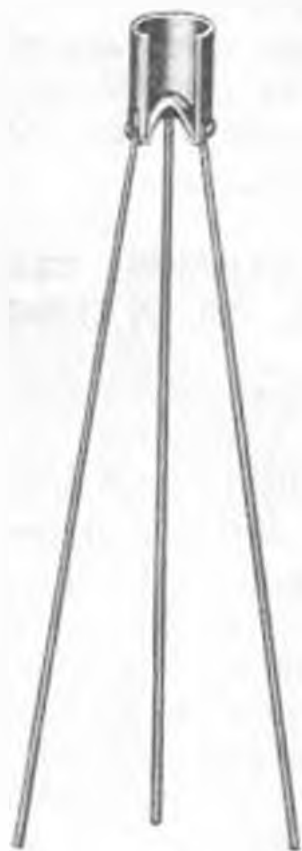
Figure 12. Container, cavity charge, Mk 2.
