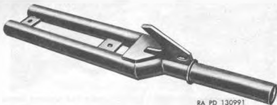
Figure 71. Nose adapter and towing hook; demolition snake M3.
