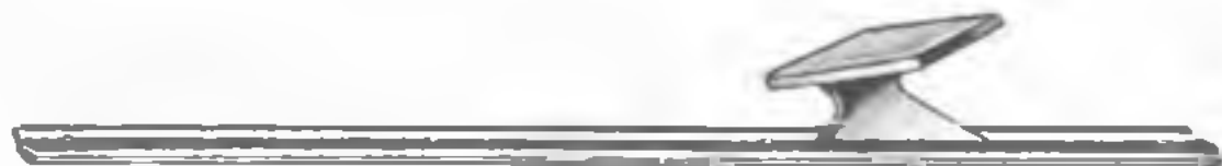
Figure 73. Pushing hook, demolition snake M3.
