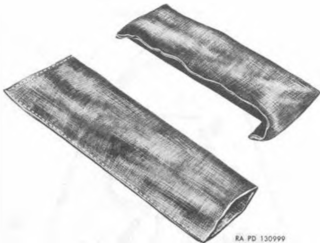
Figure 82. Tamping bags, demolition snake M3.
