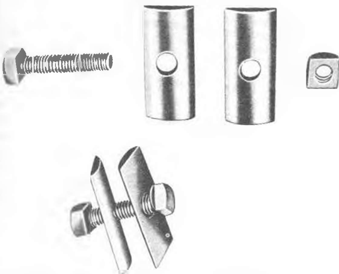
Figure 70. Bolts, washers, and nuts for demolition snake M3.
