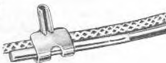
CONNECTING BLASTING CAP TO CORD
