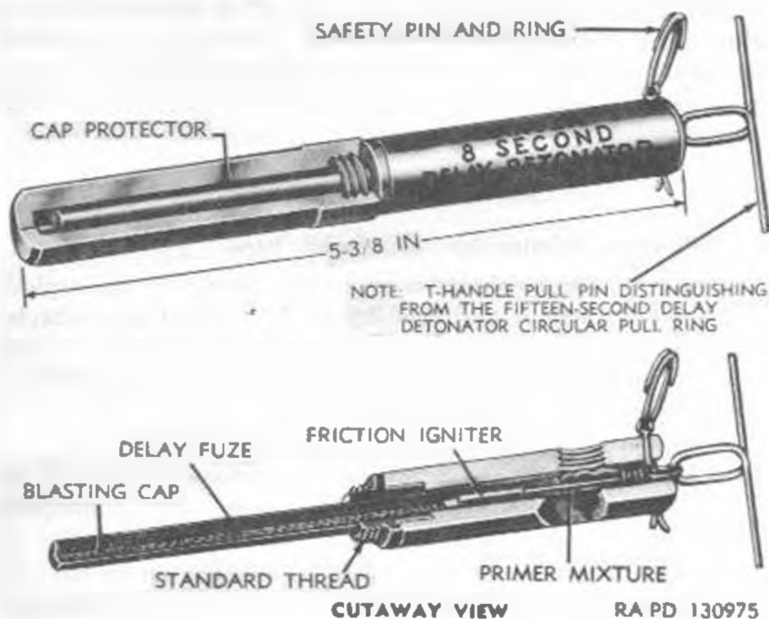
Figure 17. Detonator, 8-second delay, M2.
