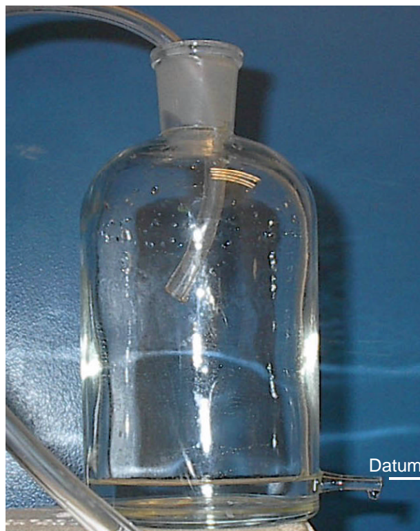
Figure 2. The model reservoir showing the no flow condition used as an elevation datum .
