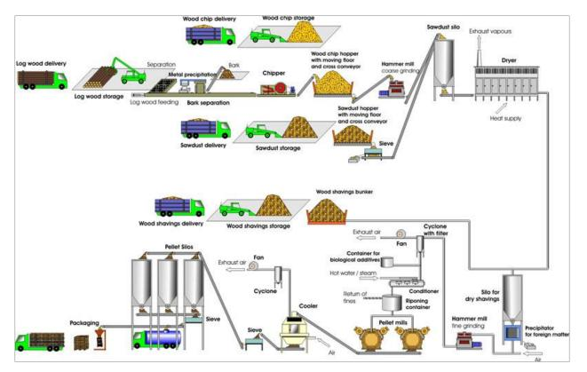
The following schematic provides a visual perspective of a pellet mill.
