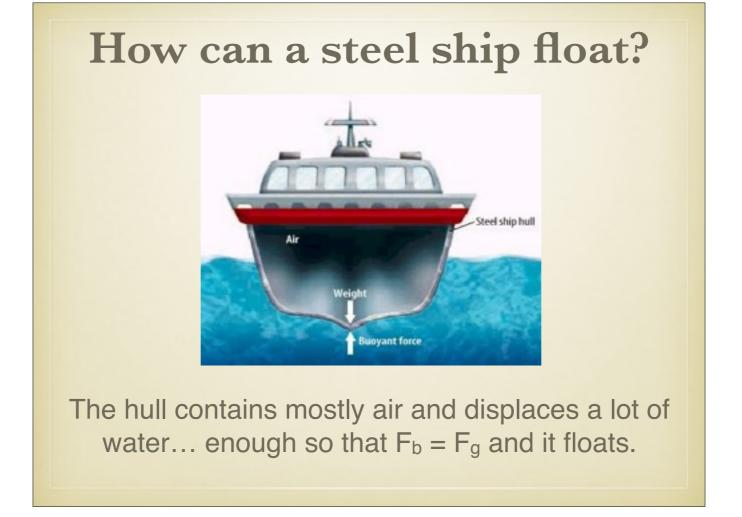
Average density of the ship (including air) is less than water.
