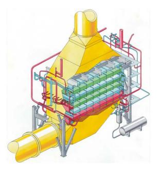
Fig. 2: Sketch of a vertical type HRSG [27]
