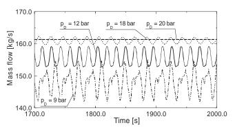
Fig. 7: Mass flow in the downcomer at different drum pressures
