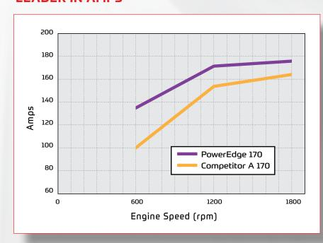
The DENSO PowerEdge patented design produces higher amps at idle and cruise speeds, allowing you to confidently, and efficiently, run all the electrical systems you need. With greater amps at idle and cruise than the leading competition, your batteries are restored quicker after start-up, and battery life is prolonged by our remote sense function.
