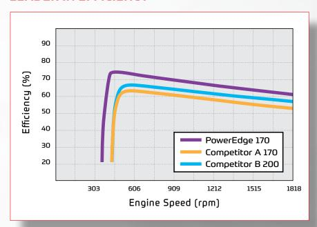
In addition to recharging your batteries more efficiently and saving you money by prolonging battery life, the **DENSO PowerEdge** is the most efficient alternator available from any manufacturer. Increased alternator efficiency means less engine power is required to operate the alternator, and that is bound to provide a savings to your bottom line when it comes to fuel expense.
