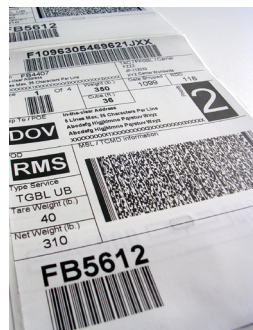
Military Shipping Label or MSL: This is the DoD label that has all the shipping and product information included.
