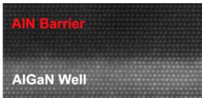
Scanning transmission electron micrograph of an AlGaN/AlN multiple quantum well 3 nm wide used for deep-UV light emitting diodes.
