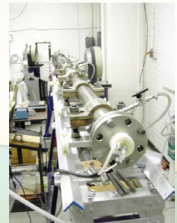
Detonation tube facility
