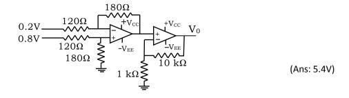
26. Calculate the output voltage for the circuit shown below.
