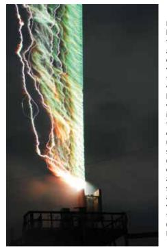
Figure 1: Triggered lightning from the tower launcher at the ICLRT. The copper triggering wire explodes at the right (straight vertical green line) with the wind blowing its remains to the left. Several downward leader/ upward return stroke sequences (tortuous white channels) follow at hundredths of a second intervals, also blown by the wind to the left in this time exposure. (Photo by Dustin Hill).
