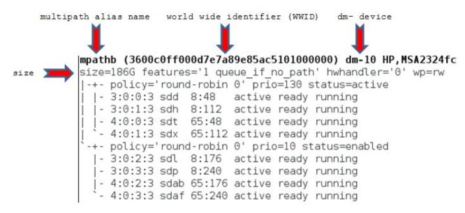
Figure 3.4.1.1: Multipath Device (mpathb)
