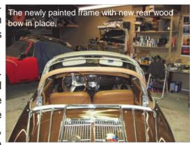
goes above the back window. The old rear bow was pretty worn out with a multitude of staple, nail and trim piece holes, several of which were in the joints in the bow on both sides where the bow curves down. The chrome aluminum strip on the outside rear of the top attaches to this wood bow. The new bow was one piece with no joints. It was cut and then steamed to get the right curvature. The new bow should be much stronger than the old one.
