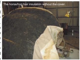
With the padding in place, the canvas top can then be installed. This requires a lot of tugging, pulling, gluing, fastening, and (to my dismay) cutting. I never thought the plastic back window would be anything but a creased and rippled piece of plastic, but after a couple of days of pulling, tugging and fitting the top, the window lost all its creases and ripples. At this point things were looking pretty good to me. I thought the project was near the end. But wait there is more.
