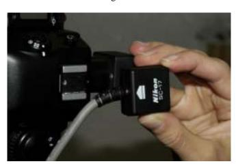
Exhibit 4-10. Connecting the IR cable to the camera
