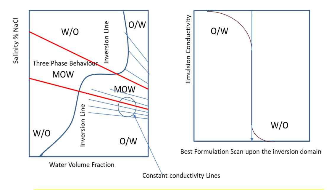
The electrolytic conductivity changes drastically inside the three phase region Indicating that the emulsion inversion takes place. The exact formulation wherein the phase inversion is located depends mostly by the Water to Oil ratio
