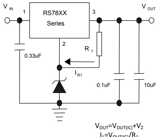
Circuit for Increasing Output Voltage
