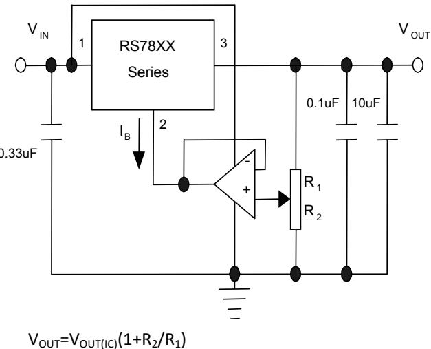
High Output Current with Short-circuit Protection
