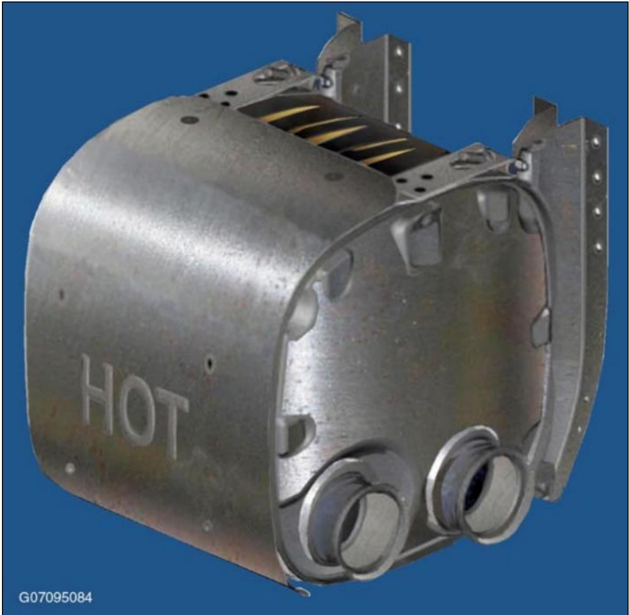
Fig 3: Aftertreatment Selective Catalytic Reduction (SCR) System Components
