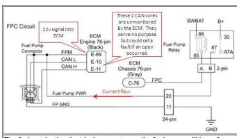
The 6 pin style, the electrical connector on the fuel pump will have 6 pins, the engine harness may be equipped with 5 wires or 3 wires.
