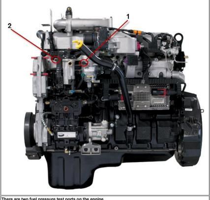
There are two fuel pressure test ports on the engine.
