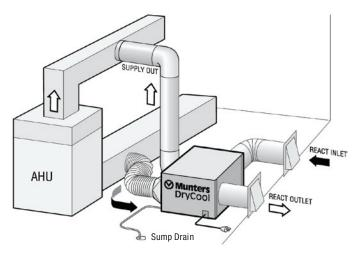
Conditioned Unventilated Basement Installation
