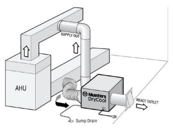
Ventilated Unconditioned Basement Installation
