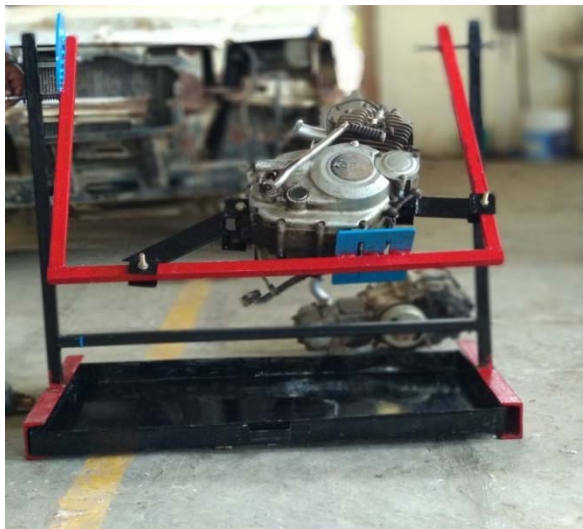
Fig 8 Final fabricated engine stand
