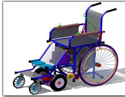
Fig. 1: Wheelchair Assembly in CATIA V5
