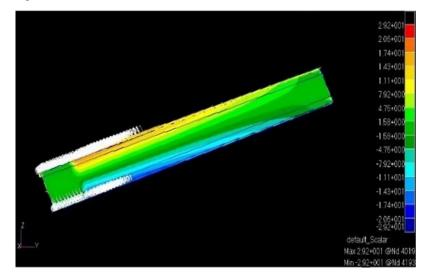
Fig. 5 Maximum stress of the spar
