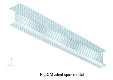
The boundary conditions are now applied to the spar model. Since the model considered is a cantilever beam, one end is fixed, ie., all the six degrees of freedom are constrained and at the free end load is applied.
