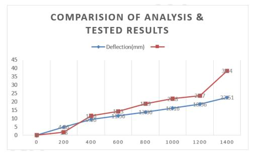
Fig 7: Comparison of Result (Load Vs Deflection)
