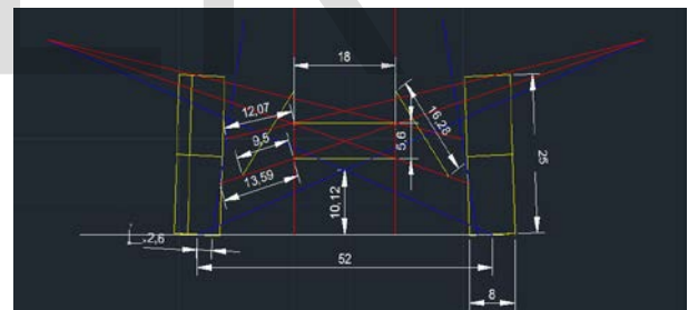
Fig 3.2: Front view of front suspension geometry
