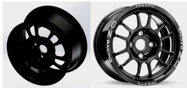
Fig 27 Rim CAD model and actual component
