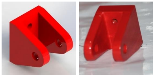
Fig 19 Lower bracket CAD model and actual component
