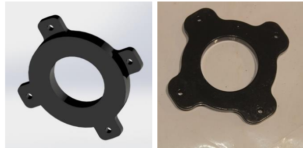
Fig 17- Bearing lock CAD model and actual component
