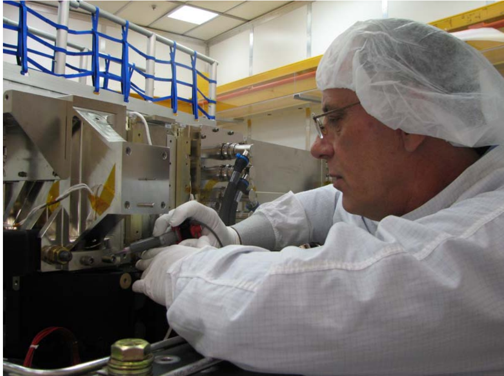
Figure 24: Coating of one of the LAT FHW Connectors using a mix recorded in the MMR Log
