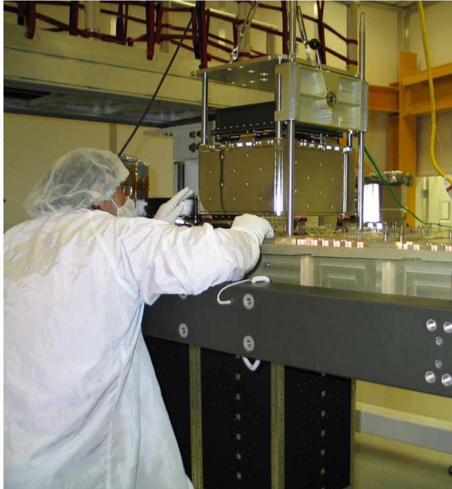
Figure 23: First CAL Module Installation into the LAT
