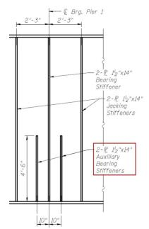
Figure 7: Auxiliary Bearing Stiffeners and Future Jacking Stiffeners at Pier 1 (shown) and Pier 4 (similar)
