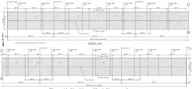
Figure 10: Plan View of Deck Placement Sequence
