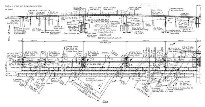
Figure 2: Plan and Elevation Drawing of the new I-270 Bridge over the Chain of Rocks Canal
