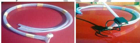
Plate 2.3c: Water distribution channel and a submersible pump (pump unit)
