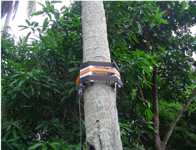
Illustration 9: Wheeled Robot Climbing a Coconut Tree [4]
