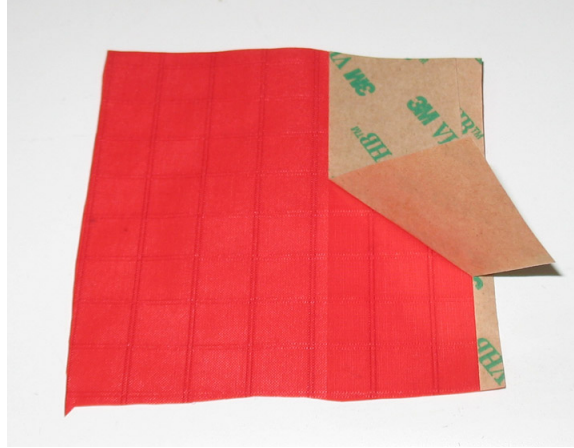
Figure 6-1: A section of the wing material with the 3M VHB adhesive tape applied.
