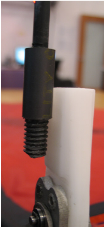
Figure 6-3: The compliant wing spar end assembly.
