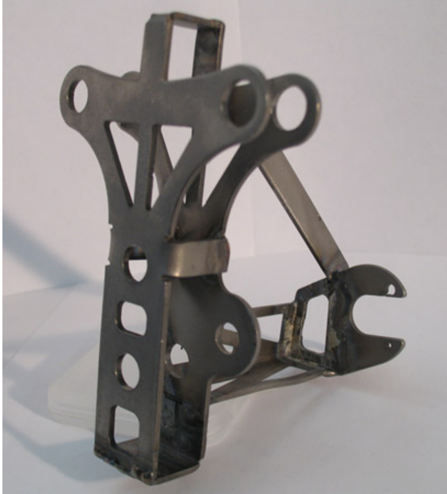
Figure 7-8: The welded titanium gearbox frame which holds all of the drive components together. Bent and welded sheet construction produces a strong, lightweight, and inexpensive part.
