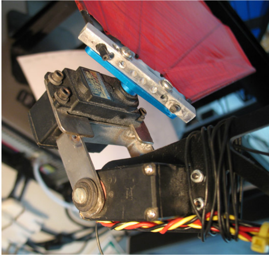
Figure 8-2: The tail section of the Phoenix. In contrast with the Kestrel the servos are directly joined in an effort to simplify the mechanism and save weight.
