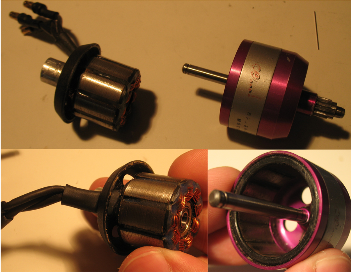
Figure 7-6: The brushless outrunner motor used in the ornithopter gearbox taken apart to show its unusual configuration. Notice that the outside can of the motor rotates rather than the coils inside.
