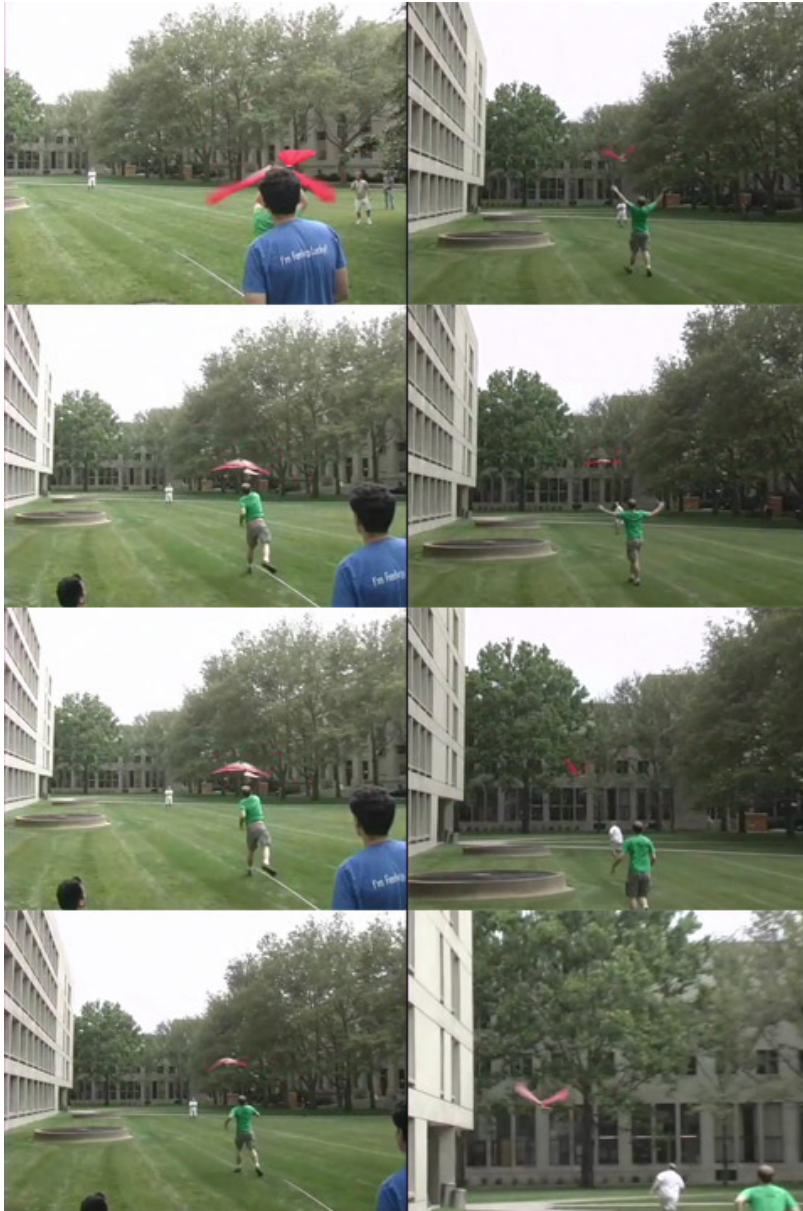
Figure 11-4: Several frames from the video of the first successful semi-autonomous flight of the Phoenix. The robot maintained steady level flight until shut off to avoid impacting the building. The author (in blue) is handling the throttle set point and controller switchover while graduate student John Roberts (green) launches the robot.
