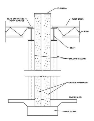
Figure 4 Back to back firewall construction. Note that the only connection is at the roof flashing.
