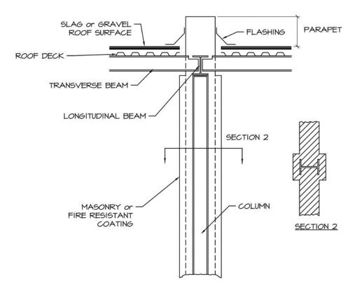
Figure 8 Tied firewall with double column or single column encased in masonry/concrete construction.
