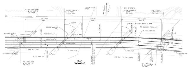
Figure 13: Span layout of Broad Run Bridge
