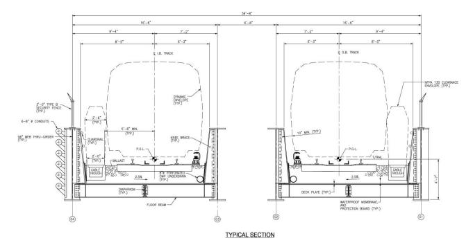
Figure 9: Typical section of Horsepen Run Bridge Page 7 of 11
