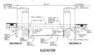
Figure 5: Centreville Road Bridge final design span configuration.
