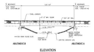
Figure 8: Horsepen Run Bridge span configuration.
