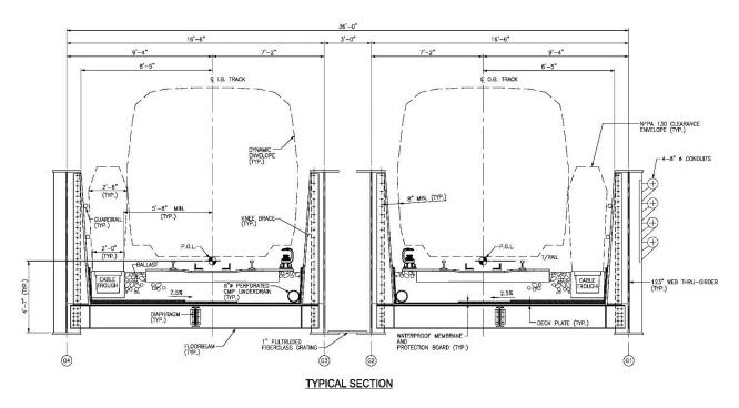
Figure 6: Typical section of Centreville Road Bridge
