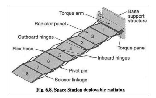
Figure 13: Deployable radiator preliminary concept (Gilmore)
