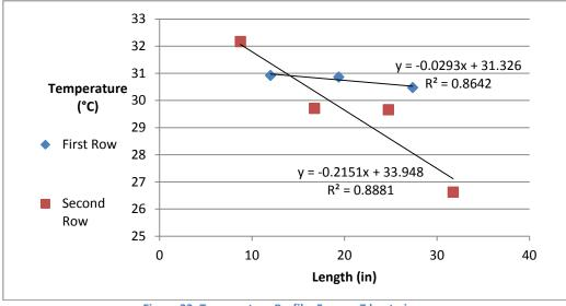
Figure 32: Temperature Profile: Fan on, 7 heat pipes
