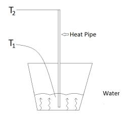
Figure 21: Heat pipe experimental set-up
