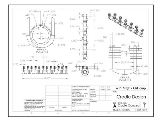
Figure 42: Preliminary design drawing, using heat pipe concept
