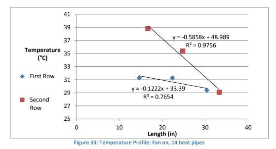
Overall, the results from the experiments with 7 heat pipes were inconsistent and led to a lot of uncertainty. The results from the experiments with 14 heat pipes were more consistent, like the ones in Figure 30 and Figure 33, and therefore more meaningful.
