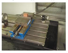
Figure 47: Securing copper for machining
