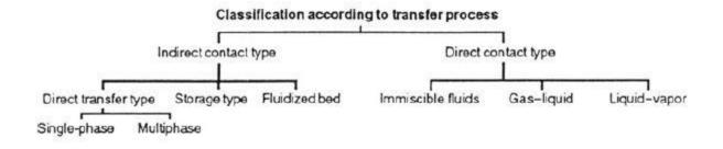
Figure 2: Heat exchanger classification according to transfer process
