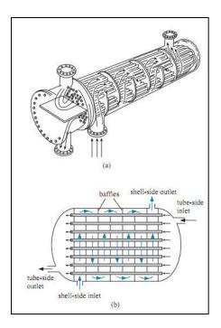
Figure 4: Shell-and-tube heat exchanger
