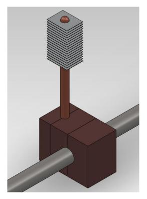
Figure 18: Cradle with Heat Pipe
