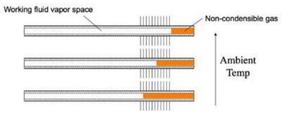
Figure 7: Variable-Conductance Heat Pipes
