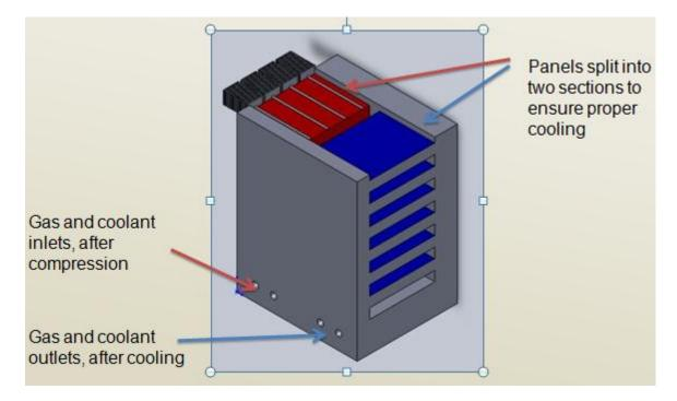
Figure 14: "Panels with heat pipes" preliminary concept
