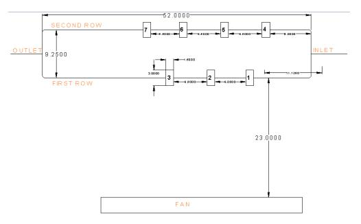
Figure 26: 7 Cradle Demonstrator Layout
