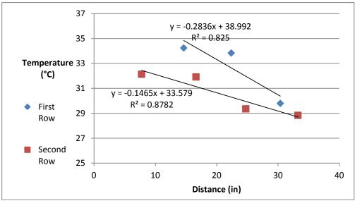
Figure 30: Temperature Profile - Fan off, 14 heat pipes
