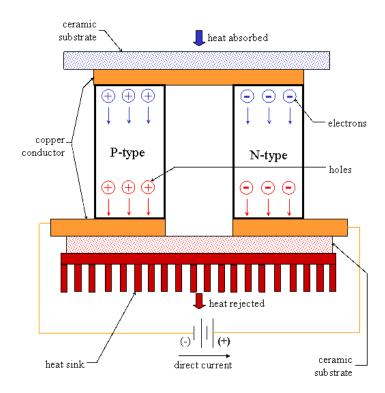
Schematic of a Thermoelectric Cooler
