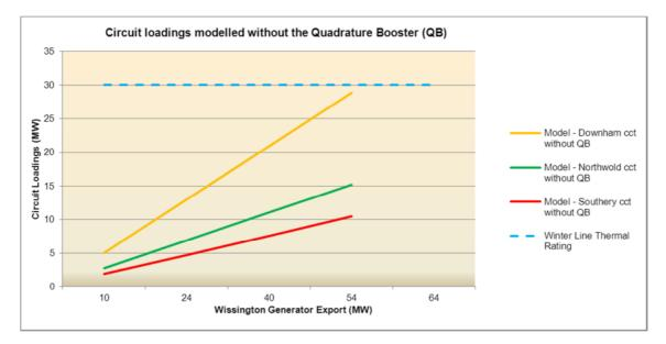
Figure 6: Modelled circuit loadings without Quadrature Booster
