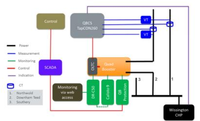
The diagram below shows simplified scheme architecture for the Wissington Quadrature Booster.
