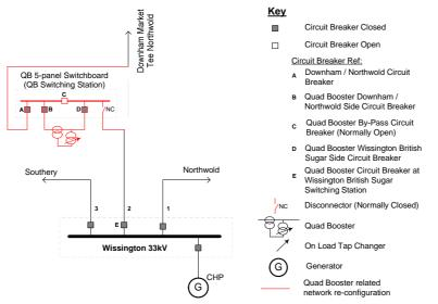
Figure 2: Simplified Single Line Diagram
