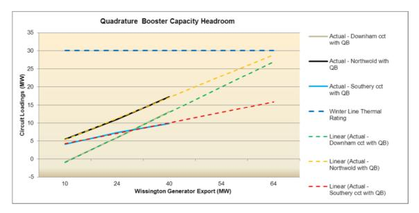
Figure 7: Graphs showing measured line loadings - and extrapolations
