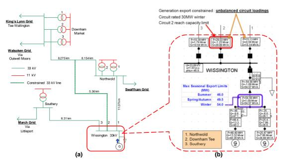
Figure 1: (a) Simplified Wissington 33kV Network, and (b) related Load Flow indications
