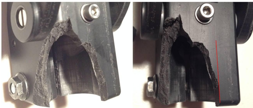
Figure 4.15: Fractured testing specimen during the initial structural testing (bottom component)
