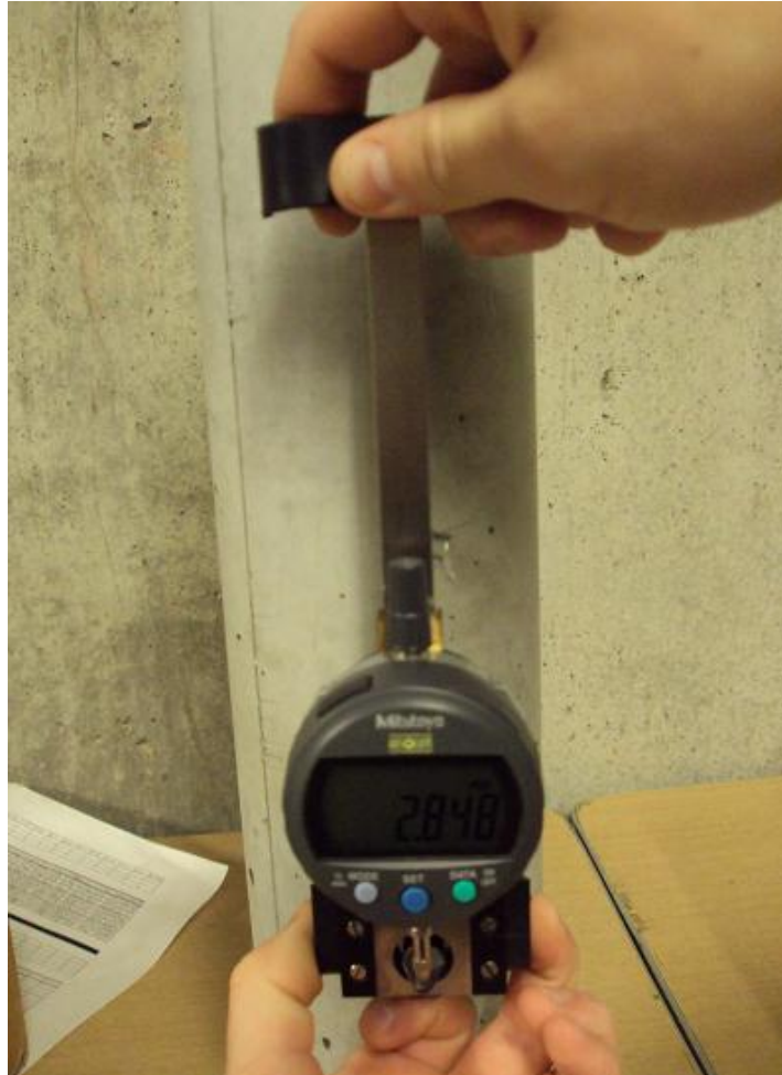
Figure 2.3 – DEMEC Reading Taken on Specimen
