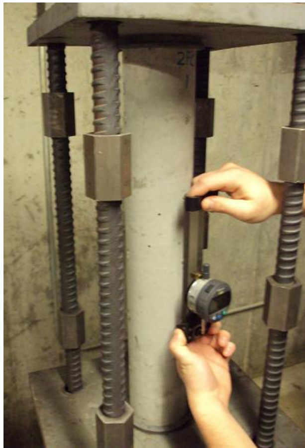
Figure 2.10 - Reading Taken on Creep Specimen
