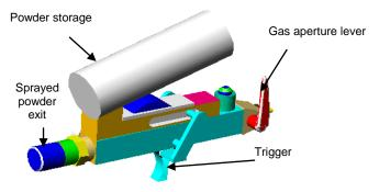
Fig 1: Spray gun, model 5PII, Sulzer Metco.
