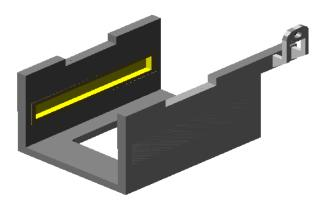
Fig.4: Housing for protection of the trigger.
