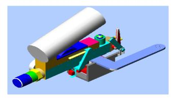
Fig 7: Spray gun with the automation system assembled.
