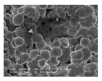
Fig15: SE Micrograph showing the structure of the coated surface obtained with ACPTSP.SEM. 200 X.
