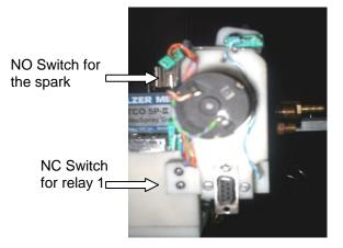
Fig 10: Geared motor coupling to the housing of the automation system.
