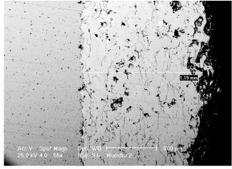
Fig 16: BSE Micrograph of the Ni-Cr-Fe-B-Si coating showing better uniformity of thickness and reduced porosity of the coated surface obtained with ACPTSP. SEM 55X
