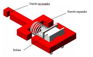
Fig 3: Shutter system for the trigger
