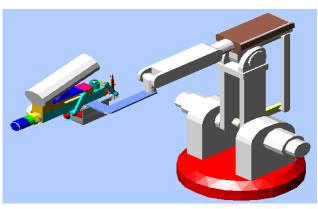
Fig 8: Robot arm with the automated combustion powder thermal spray gun attached.
