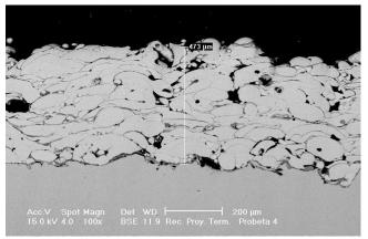
Figure 14.- SEM Micrograph of a Ni-Cr-Fe-B-Si coating obtained by a conventional manual combustion powder thermal spray process. Its possible to see limited adherence and high porosity.
