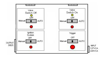
Fig 11: Control Box distribution
