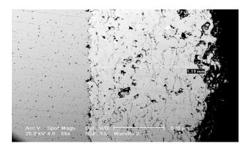
Figure 12. Image of coating of NiCrFeBSi obtained by flame thermal spray on AISI 1018 carbon steel. Thickness of 1.19 mm height of the layer. SEM. BSE
