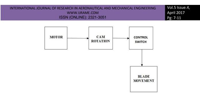
Fig 1.1 Block diagram of cutter arrangement
