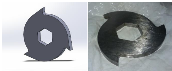
Fig 6:- Blade Model and Manufactured Sample
