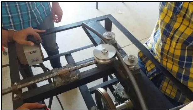
Figure 3.1 Setup of machine for rolling operation
