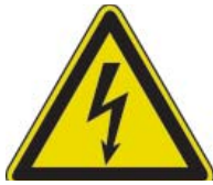
Warning of dangerous electric voltage
