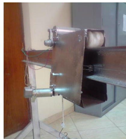
Fig. 15. Prototype trolley mechanism (derived by two DC motors)
