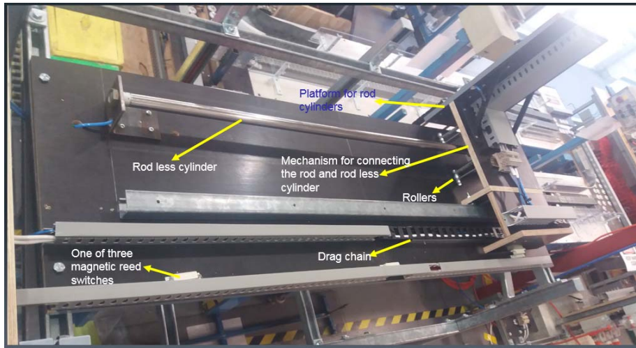
Figure 32: Top view of the pick and place device
