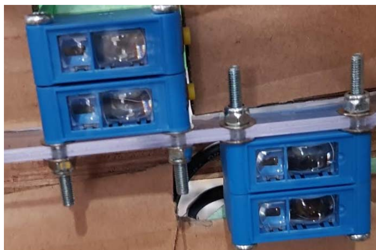
Figure 9: CSM-WP117A2P colour sensor
