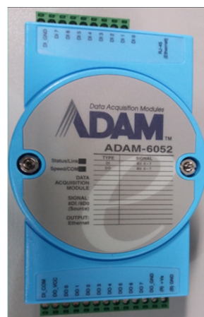
Figure 16: ADAM 6052 I/O module with specifications (ADVANTECH Co. Ltd, n.d.)
