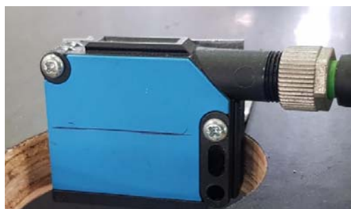
Figure 8: WL11-2N2430 retro-reflective sensor
