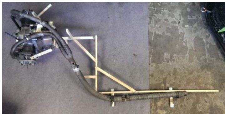
Figure 18: wooden structure to produce the new exhaust with the old exhaust installed
