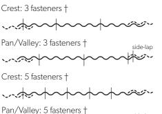
† Fasteners per sheet per support. Most common practice is: 3 fasteners for internal spans and 5 fasteners for single and end spans.
