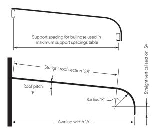
Span to be used in determining wind pressure capacities of bullnoses
