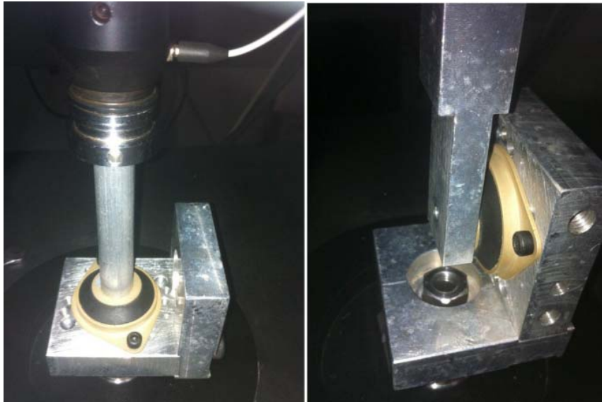
Figure 8.29 Axial (left) and radial (right) test configurations of the prototypes
